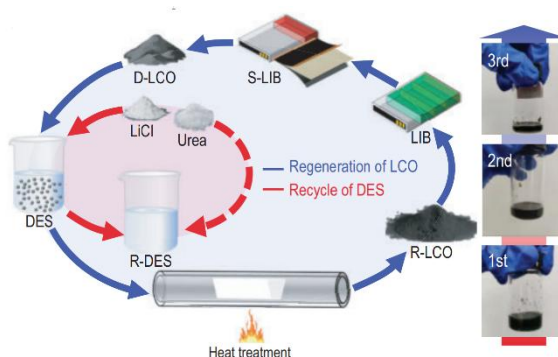
Figure 15: Eutectic solvent use cycle [74]
